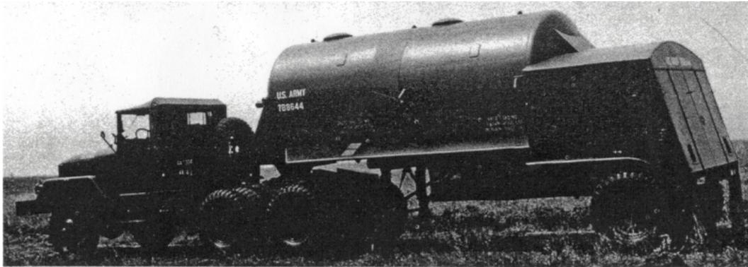
Figure 39. Each firing battery has two liquid oxygen (LOX) semitrailers that carry the oxidizer to service the missile. Each trailer can hold 9 tons of LOX. The trailer has a "thermos bottle" construction to maintain the LOX at a temperature of minus 297 degrees Fahrenheit. The LOX transfer pumps and equipment are mounted in the closed compartment at the rear of the trailer.
