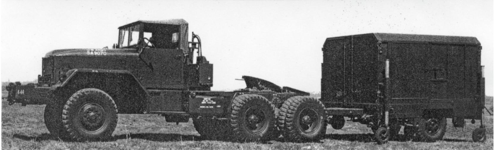
Figure 24. The aft unit is transported on the XM480 trailer. Like the other two trailers, the upper portion or cover of the trailer is removed by lowering a set of four extendable legs (shown in bottom photo). The cover is then elevated by a series of jacks and the entire assembly is pushed to the rear by battery personnel thereby uncovering the aft unit.
