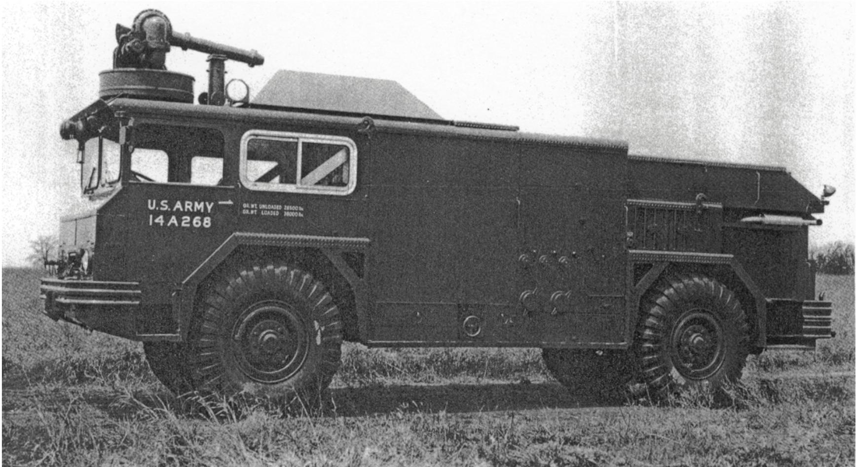
Figure 41. The fire truck carries 1,000 gallons of water and is used to neutralize spilled propellant or to extinguish small fires which may ignite when the missile is fired. The truck normally tows a four-wheeled water trailer which contains a 2,000-gallon reserve.
