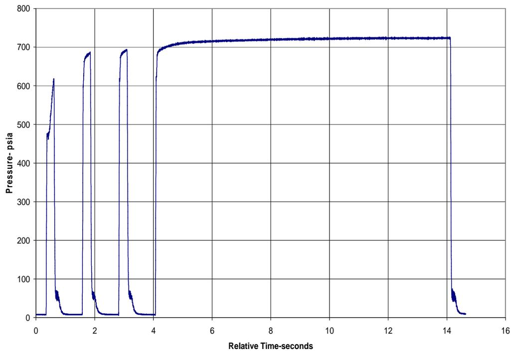
Figure 4. Example Measured Pressures for Flux  $\sim 1.4 \text{ lbm}/(\text{in}^2\text{-s})$ ,  $P_c \sim 725 \text{ psia}$ ,  $C^*$  Efficiency 95%
