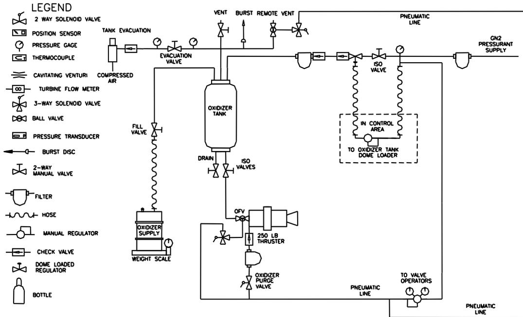
Figure 1. Schematic of Test Stand and Article
