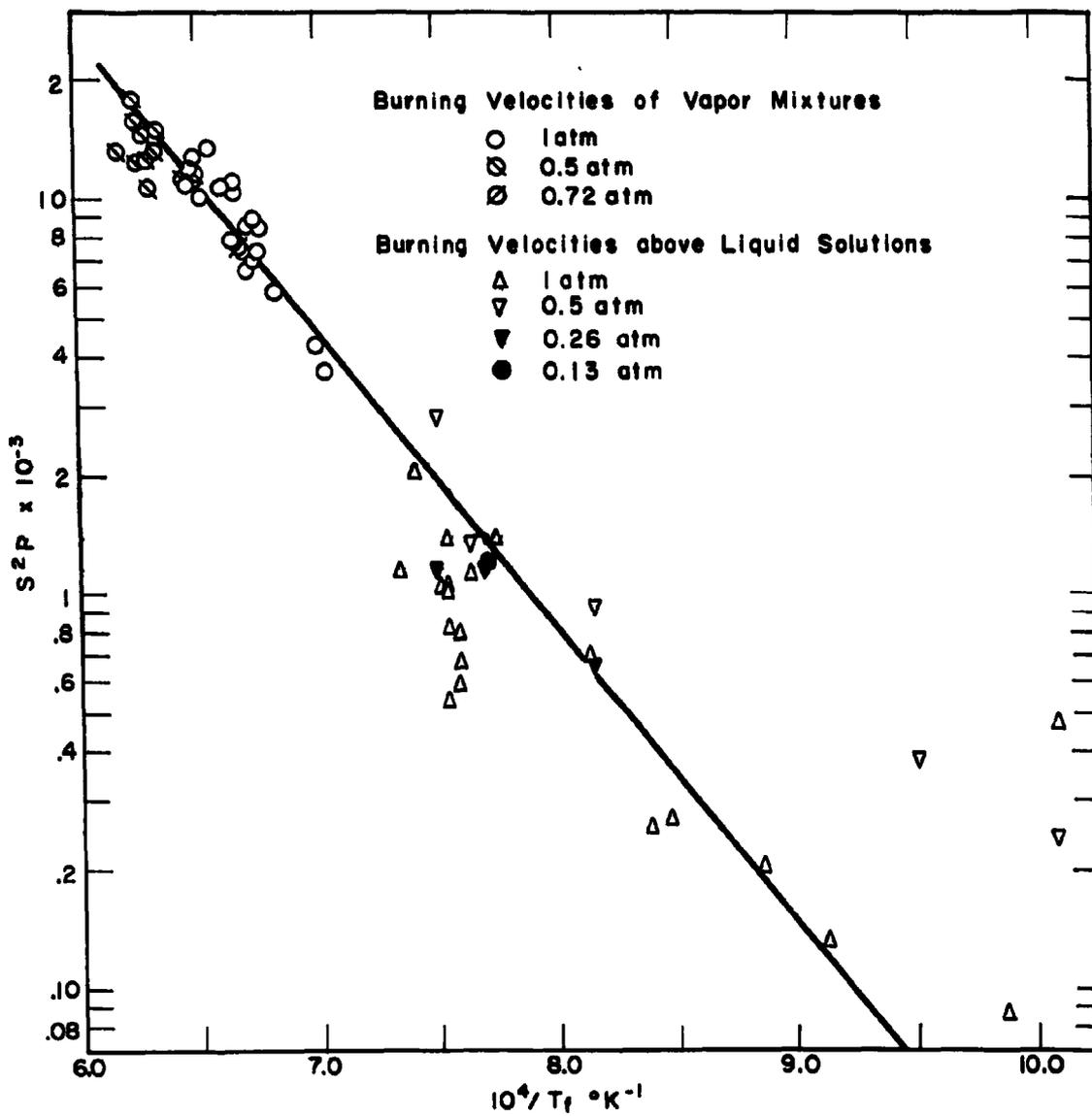
FIG. 8 CORRELATION OF BURNING VELOCITIES OF VAPOR MIXTURES AND LIQUID SOLUTIONS OF  $\text{H}_2\text{O}_2$
